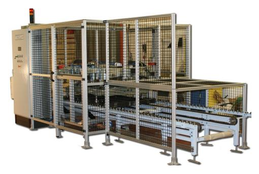
TQC have designed and manufactured a fully automatic solution to provide the final leak test to ensure an automotive battery tray is fit for purpose.
