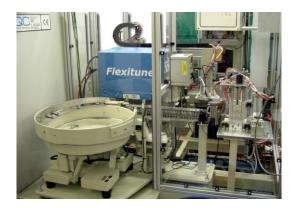
Temperature, load and position monitoring are used to ensure correct press assembly. Assembled parts are located by the press top tool and released onto a advancing outfeed conveyor.
