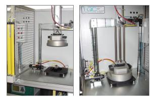
The operator manually loads a part into the machine and connects the test line to do it.
