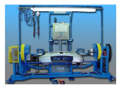
This range of equipment enhances the scope of assembly and checking fixtures to include integrated testing of fitted electrical parts such as lights and PDC's.
