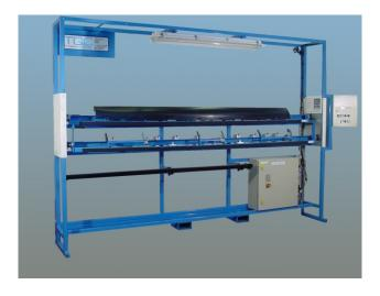
Other machines have been produced for checking the presence of manually inserted clips into Automotive body trim mouldings.
