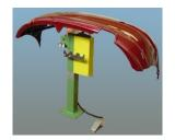
All cradles firmly support the moulding which is held in place by a dual vacuum circuit holding on the B face.
