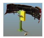
TQC polishing fixtures allow the painted moulding to be firmly held anywhere within its envelope, giving the operator the optimum working position.
