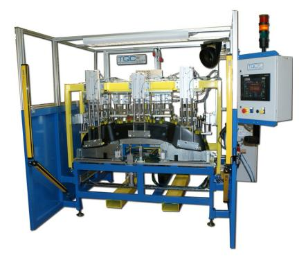
The machine tooling provides location for the main painted front bumper mouldings to which the operator adds a number of trim pieces.
