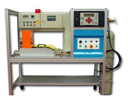
This piece of equipment has been designed and built to leak test an automotive fuel rail to a leak specification limit of 4mm<sup>3</sup>/sec at 3.5 bar.
