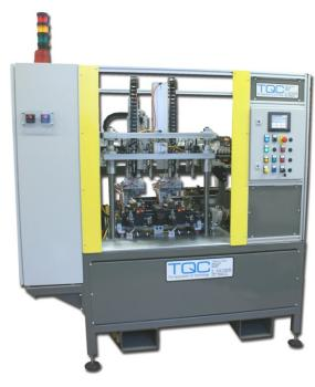
This machine was produced for an automotive plastics moulding manufacturer to automatically insert 6 threaded brass inserts and 3 steel compression limiters into a Throttle Body Moulding.
