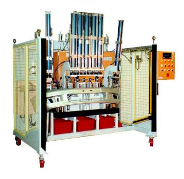
The photo below shows how TQC linked an air test facility with an automatic insert placement operation enabled a simple quality control function to be incorporated into the process—inserts were only fitted to components which passed the leak test.
