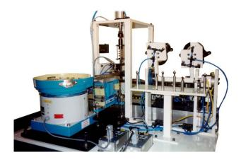
The facility shown above, incorporated component movement mechanisms, pick & place devices, servo-position driven actuator and ultimately the punch unit which drives inserts into mouldings two at a time, before being discharged from the machine.
