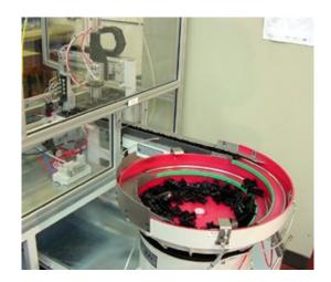
The facility is completely guarded with aluminium extruded frames and clear guard panels. All of the openings for the bowl feeders are outside the guarded area, allowing the operator to top up the bowls without stopping the machine. The deposit point for the assembled and tested product is also outside of the guarded area. The carton filling system also has an automatic carton change facility.
