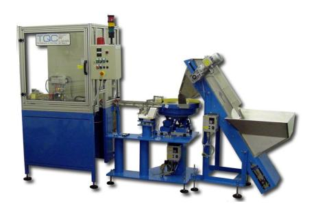
TQC designed and manufactured a standalone machine for the automatic feeding and checking of an automotive plug.
