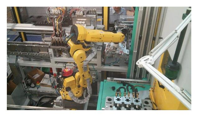
This robot cell includes automatic handling, component bowl feeding, automated leak testing, passed and failed part segregation and automatic packing of automotive moulded plastic sensors.
