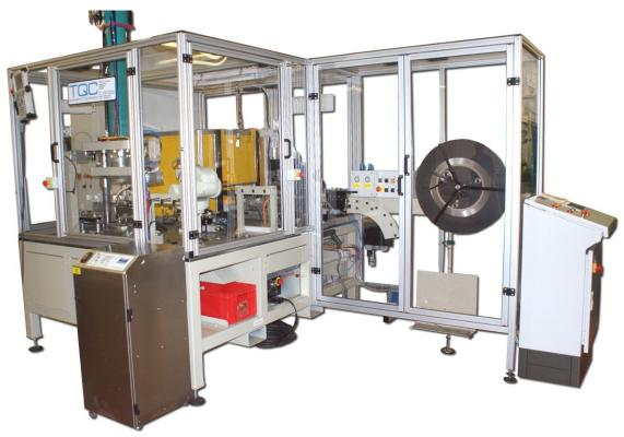
The system incorporates multi stations that perform individual tasks to complete the manufacturing process, with a Kawasaki 6-axis robot being used to move product between the various manufacturing stations.
