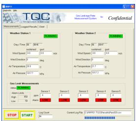
The specific application was for a submarine with the system used to monitor the flow characteristics within the vessel and how this was affected by the weather conditions outside when the submarine was at the surface and the hatch was open.
