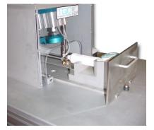
The machine was designed to leak test the inductance weld on a plastic shower head.
